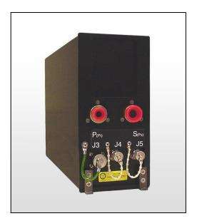
The 9B-81050-3 DADC replaces the SAT/TAS/TAT computer, as well as the altitude and airspeed sensors on the C-130 aircraft. Air data information is provided digitally to onboard systems, including flight management and navigation systems, through dual MIL-STD-1553B and dual ARINC 429 busses. Continuous BIT insures the integrity of all data provided.
