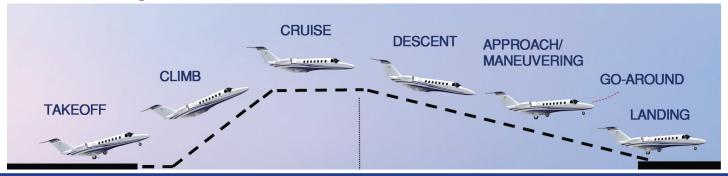
**TAKEOFF MODE:** ThrustSense® is engaged for takeoff. ThrustSense will automatically advance the Throttle Levers to the takeoff detent.
