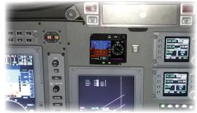
The Integrated Standby Unit houses the computer that controls the movement of the throttles. This elegant solution is minimally invasive and allows for a short downtime for installation without structural modifications to the throttle quadrant.
