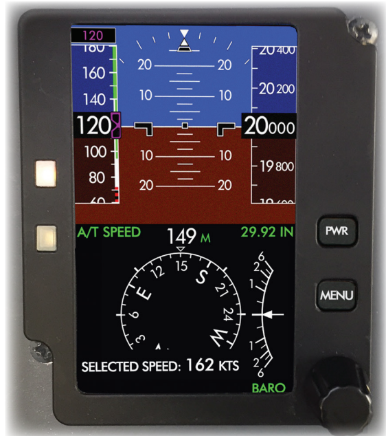
Standby Instrument commands the actuator assembly which physically moves the throttle
