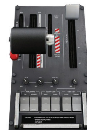
Standby Instrument commands the actuator assembly which physically moves the throttle
