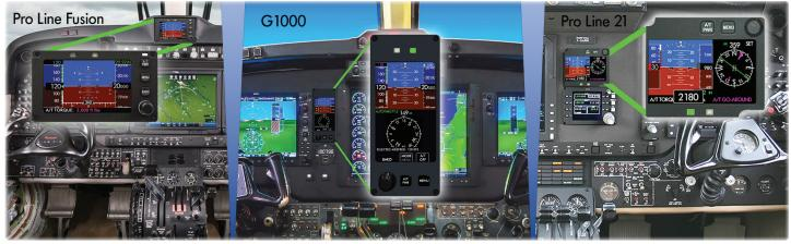
The ThrustSense® Autothrottle is commanded by the Standby Display Unit that serves as the pilot's interface mode for speed and torque selections, and also serves as a standby EFIS system. The Standby Display Unit houses the computer, which controls the Actuator Assembly which physically moves the throttle.
