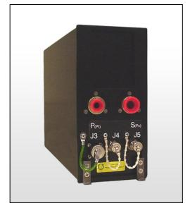
The 9D-81050-3 DADC replaces the SAT/TAS/TAT computer, as well as the altitude and airspeed sensors on the C-130 aircraft. Air data information is provided digitally to onboard systems, including flight management and navigation systems, through dual MIL-STD-1553B and dual ARINC 429 busses. Continuous BIT insures the integrity of all data provided.
